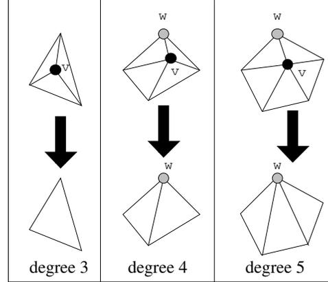
**Lemma 4.1** Let  $G = (V, E)$  be a maximal planar graph with  $|V| > 4$  and let  $v$  be any reducible vertex of  $G$ . Applying the reduction of  $v$  again results in a maximal planar graph.
